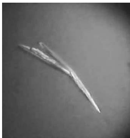
Figure 2 Crystals of the RTP-C110S-sRB complex. The plate-like crystals have approximate dimensions 0.5 \times 0.2 \times <0.01 mm.
